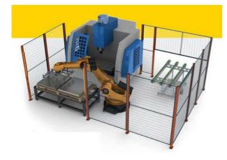
Any person entering the area enclosed by shields must protect themselves against accidental closure in the area in accordance with the provisions of the safety instructions for machinery, equipment and installations during an intervention hereinafter referred to as LOTO, by putting an individual padlock. The padlocks are provided by the Contractor, but in a crisis situation by the UR or the FT Service.
